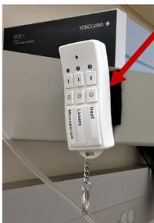
Turn on the Lasers and Microscope, Heat if needed
