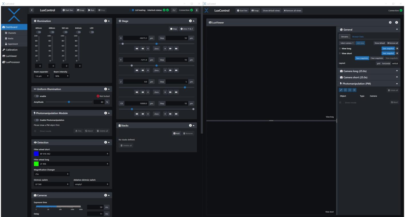
The illumination panel has the 4 different laser lines and the LED option. The beam intensity can be controlled between 10% or 90%. The beam expander controls the NA of the illumination objectives. This will have an effect on the characteristics of the Light Sheet.
