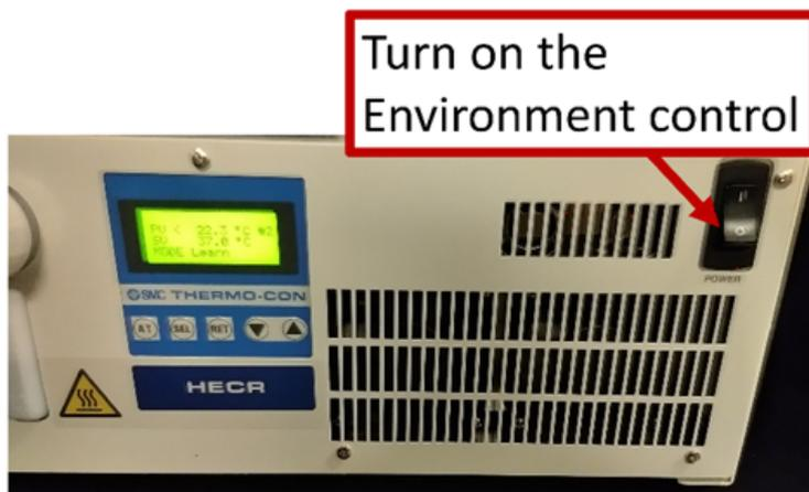
You can choose between Learn Mode or Normal Mode. The PV value is the temperature of the Peltier module and the SV value the set value of the temperature required inside the sample chamber. You will typically put the SV value at 37C.
